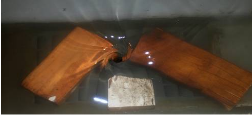
Photo 4 Orifice flow through Model Vane Grate
